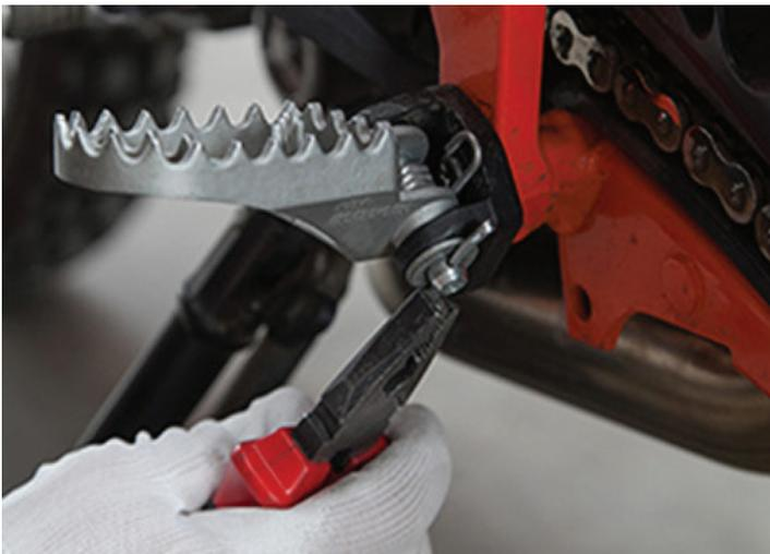
2. **Highly recommended that you wear safety glasses!** Next, you'll have to remove the Clevis pin. Be very careful, torsion spring may come flying at you, so make sure to place one hand over the foot peg bracket.
