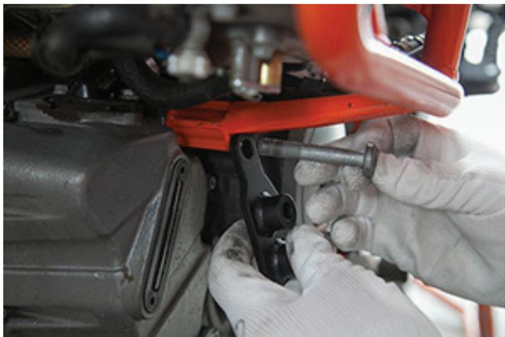
8. Remove the torx bolt from the bottom of the rear brake master cylinder. **Make sure to replace this bolt after step 17!!**
