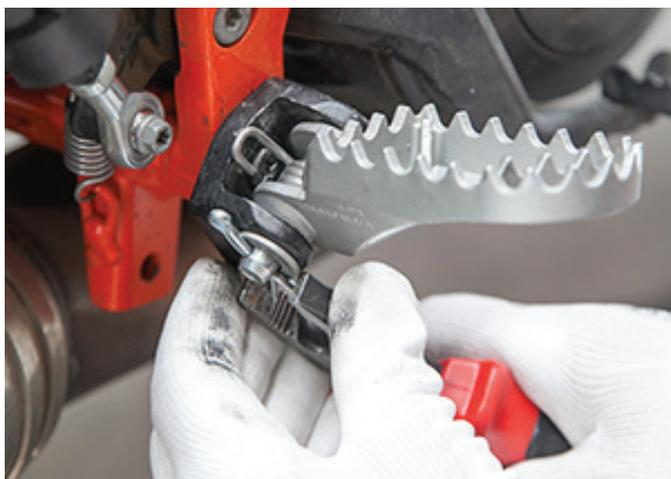
10. Mount the right side rear skid plate mounting bracket. Insert the supplied engine through bolt, hand thread it and leave it loose.
