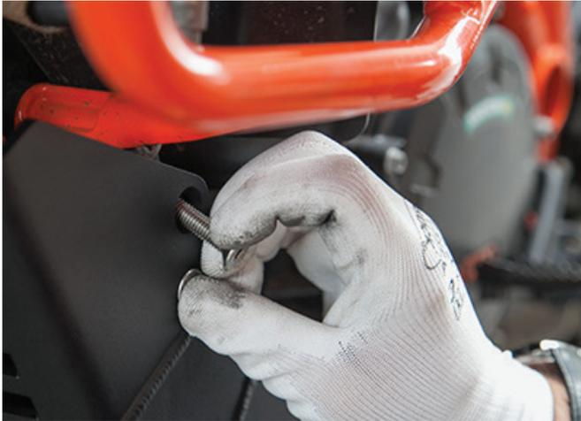
16. Insert the 8mm diameter Allen bolts through the left side rear mount. Thread the supplied nyloc nuts on the end. Leave it loose.
