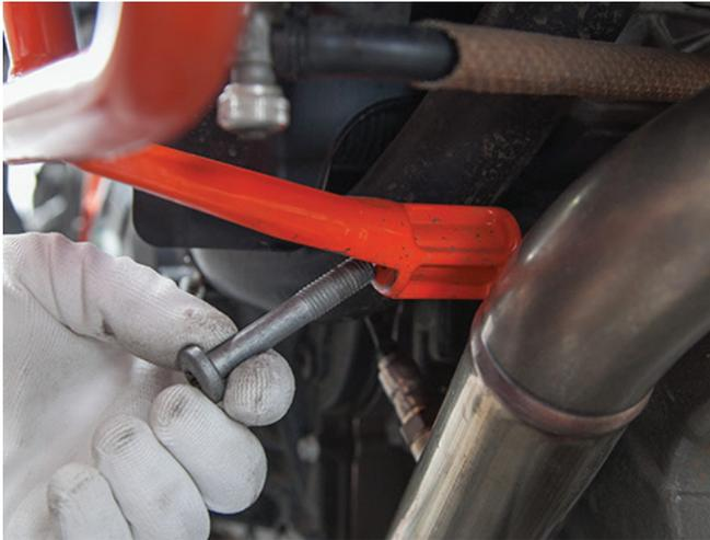
12. Mount the right side front skid plate mount (short piece). Replace the factory engine mount bolt. Leave it loose for now.
