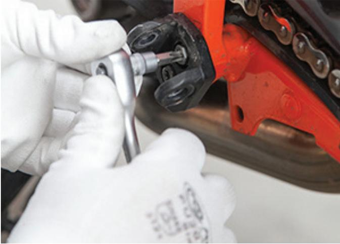
4. Mount the left side rear skid plate mounting bracket. Insert the supplied engine through bolt, hand thread it and leave it loose.
