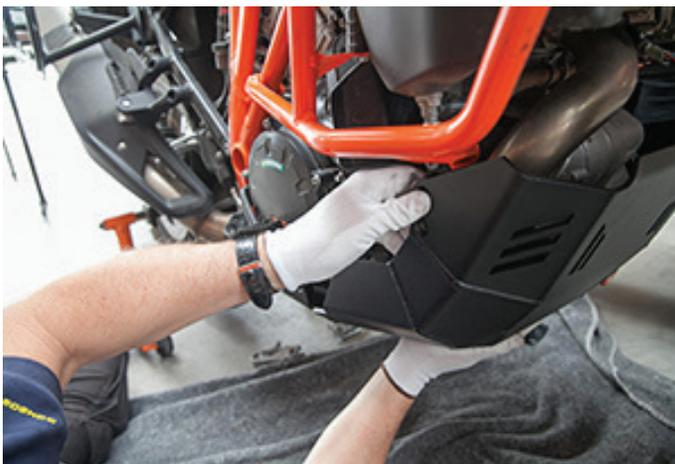
14. Insert the 8mm diameter Allen bolts through the right side upper mount. Thread the supplied nyloc nuts on the end. Leave it loose.
