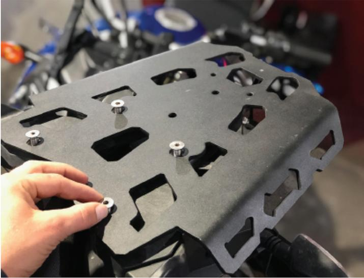
4. Take a 5mm Allen key or Allen socket and a ratchet and tighten down all four bolts.
