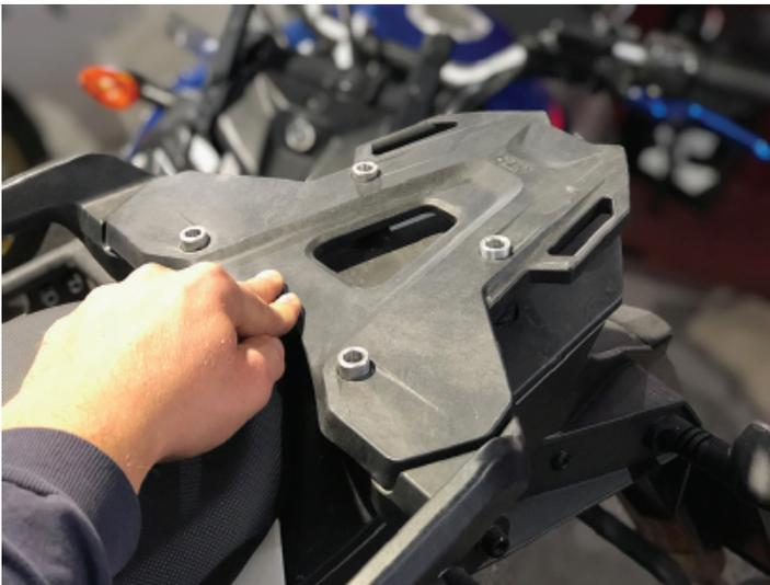
2. Next, take the rear luggage rack and gently put it on top of the four spacer. Make sure the mounting holes all line up.
