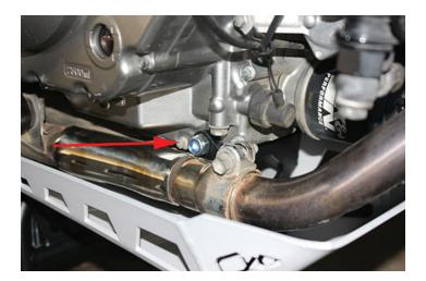
8. Using one hand align the mounting holes on the skid plate and the rear mounting bracket. Insert the M8x20mm (x2) flat head bolts into the holes and tighten both of them to the required torque. Apply thread locker.
