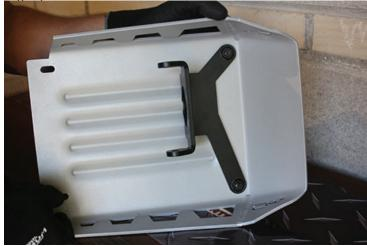
6. Insert the M10x120mm Allen bolt on the left hand side (rider's side) through the engine mount hole. Thread in the nyloc nut from the right hand side by hand.
