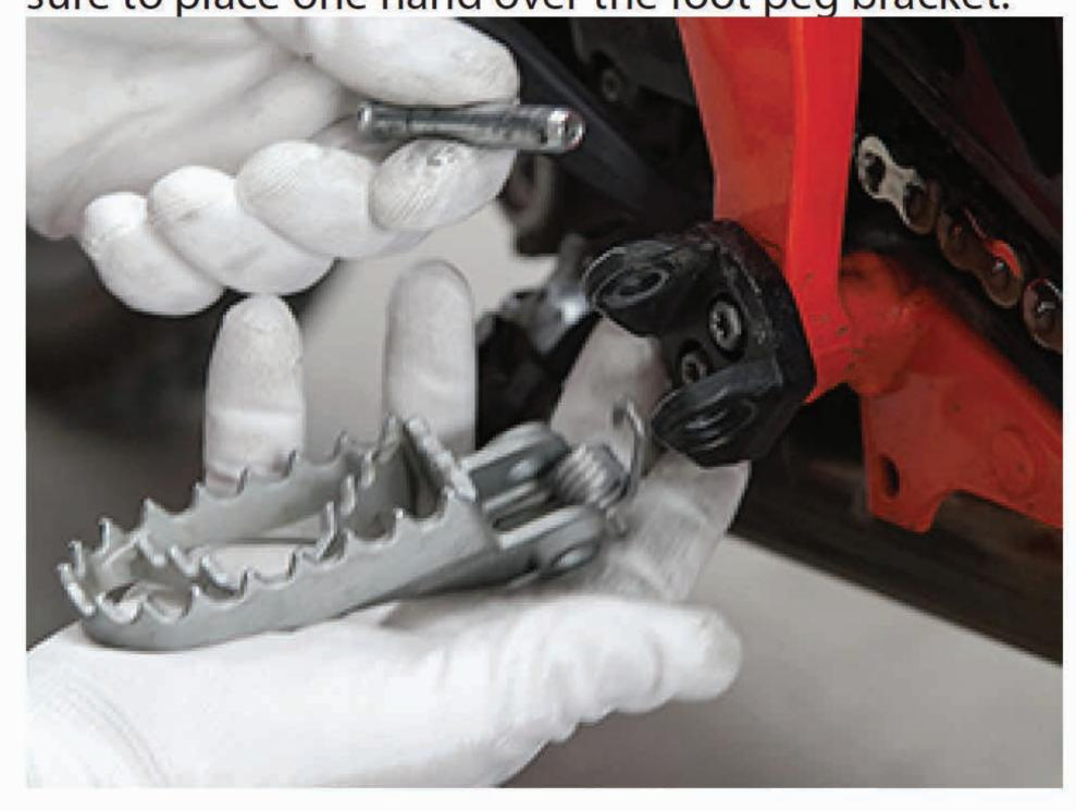
3. Remove the foot peg bracket bolts. T30 torx (?)
